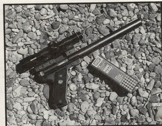
The suppressor has been designed to use high velocity ammunition and still be very quiet without a substantial drop in velocity. The author used CCI Mini Mag ammunition throughout the test with optimum results.
