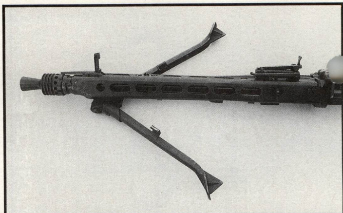
The MG42's front and rear sights fold down when not in use to protect them and to lessen the chance of getting caught on brush or clothing. The M60's rear sight folds down, but the front does not.
